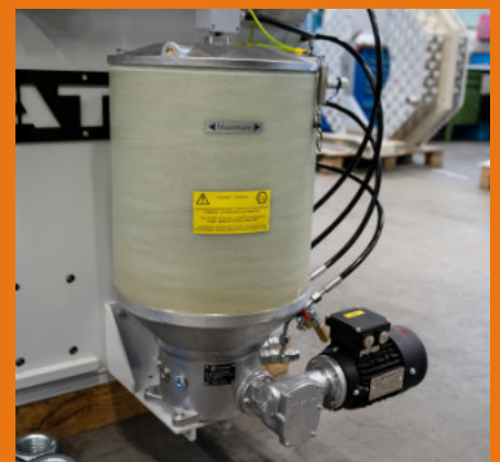
Piston pump GMF with pressure relief valves and distributors, designed for safe, efficient pellet press lubrication, with easy refilling and integrated filtration.
