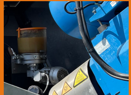
Under weather protection hood: GMA for bearing lubrication on the screw drive
