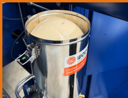
Fast and clean filling of central lubrication systems
