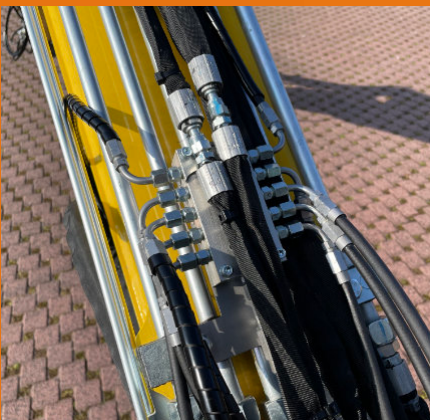
Progressive distributor serving a lubrication gearwheel
